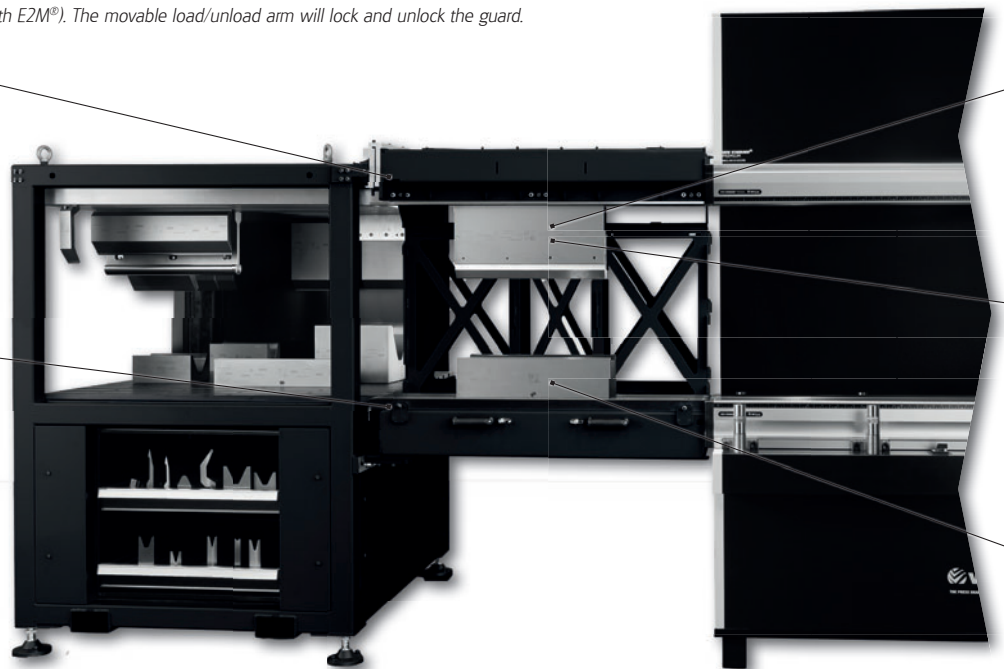
Each upper Tool Holder, used in combination with a Press Brake Productivity ToolStation, requires a dedicated guard with a safety mechanism for safe loading and unloading of the top tools (with E2M ® ). The movable load/unload arm will lock and unlock the guard.
